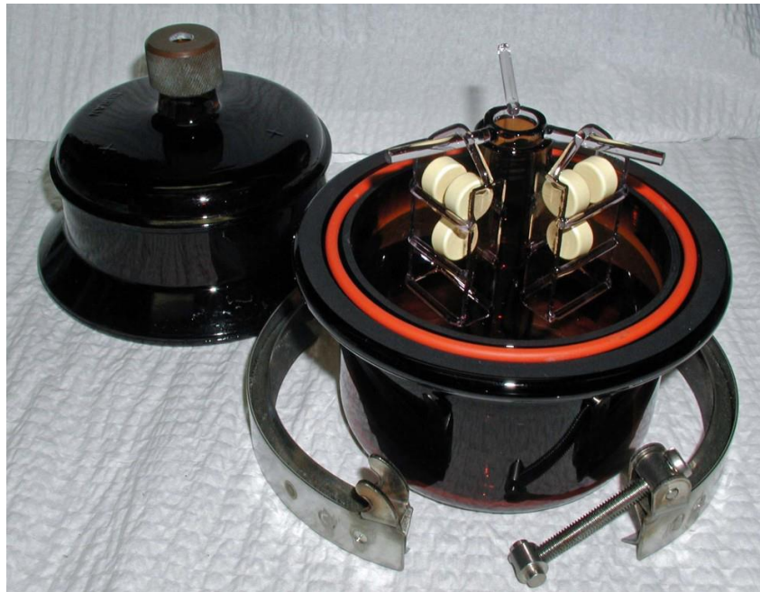
Fig. 62. Vessel for organic iodide studies with samples after irradiation [214]
